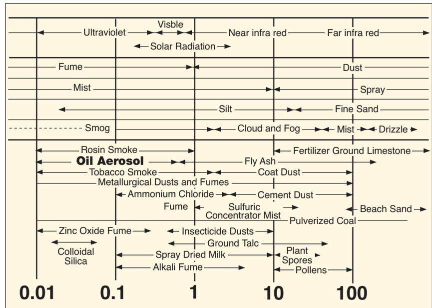
To assist in understanding the parameters of filtration, refer to this pollution size comparison chart. Look at the size of a major contaminant, oil aerosol! It is in the region of 0.01 - 0.8 micron. Tobacco smoke is also a liquid
