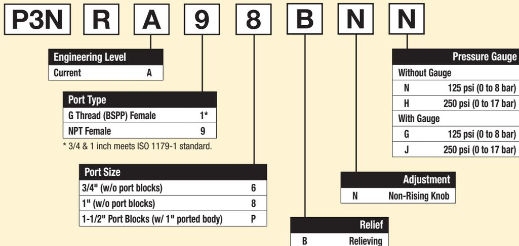
Note: BSPP ported units supplied using NPT ported bodies and BSPP port block kits.
