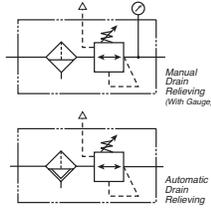
Integral Filter / Regulators are an excellent choice where accurate pressure regulation and high moisture removal efficiency are required in a space saving package.
