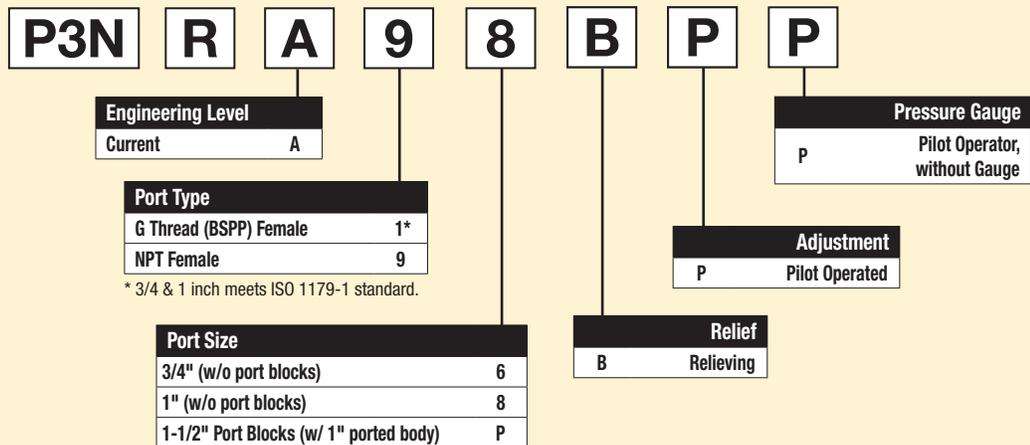
Note: BSPP ported units supplied using NPT ported bodies and BSPP port block kits.
