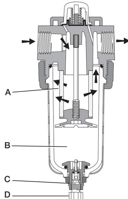
and sub-micron particulate matter. Collected liquids and particles in the “quiet zone” should be drained before their level reaches a height where they would be reentrained in the flowing air. This can be accomplished by the manual drain (C) which is actuated by twisting knob (D) counterclockwise. On the 30 Series, unscrew the drain valve (E) slightly until the liquid begins to drain.
