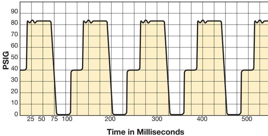
Actual test results show rapid response on a robot welding operation at a major U.S. automotive manufacturer.
