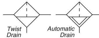
Air filters are designed to remove airborne solid contaminants, pipescale, rust, pipe dope, etc., which may plug small orifices or cause excessive wear and premature failure of pneumatic components.
