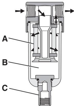
The contaminated air enters the element interior and is forced through a thick membrane (A) of "borosilicate" glass fibers coated with epoxy. Flow then passes through the element, and at this stage 99.97% of the sub-micron particles have been removed from the air stream. The tiny droplets coalesce together and are collected from the filter element by the outer drain layer.
