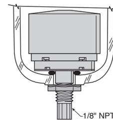
The float internal to this drain rises with increased liquid level. When the float rises, it opens a seat area allowing the trapped liquids to drain through the bottom. A manual override can be pushed in the bottom of the drain to unseat the float if particulates create a block.
