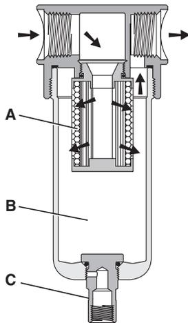
The contaminated air enters the element interior and is forced through a thick membrane (A) of "borosilicate" glass fibers coated with epoxy. Flow then passes through the element, and at this stage 99.9997% of the sub-micronic particles have been removed from the air stream. The tiny droplets coalesce together and are collected from the filter element by the outer drain layer.
