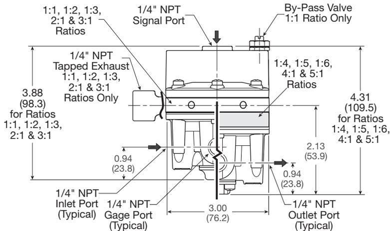
**Precision Pneumatic Input Signal Amplifier Regulator Products**
