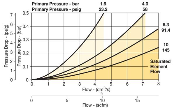
**P31 - 0.01 micron flow Coalescing Filter**
