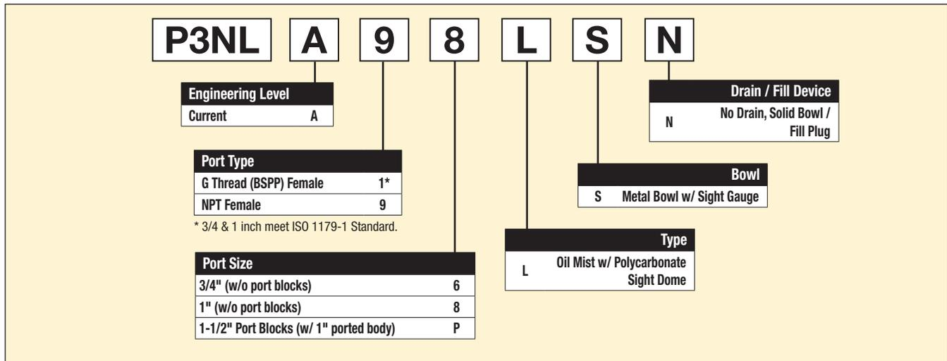
**Note:** All configured BSPP ported units are supplied using NPT ported bodies and BSPP port block kits.
