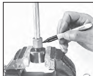
Step 6 – Make reference mark on nut and tube.
