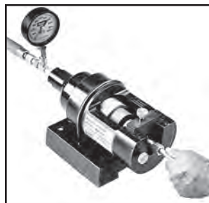
Fig. R29 — Flaring with Hydra-Tool
